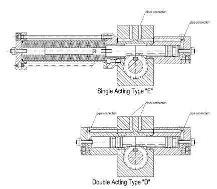
All variants are available with double-acting type D, or single-acting with spring package type E (spring opening or spring closing).
